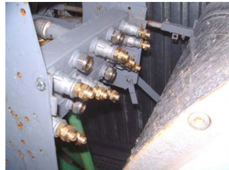
Photo 2 Below, Nozzle configurations for experiment with three rows of flat jet nozzles.
